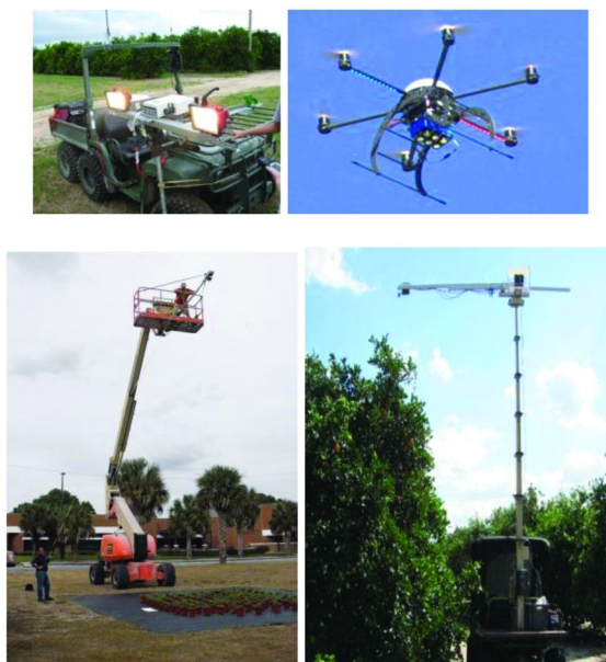
Figure 1. Sensor platforms. (a) Sensors mounted in front of a utility vehicle, (b) sensors mounted on a retractable mast connected to an agricultural vehicle, (c) high-lift platforms attached to a vehicle, and (d) unmanned aerial vehicle (not to scale). [Source: Reza Ehsani]
